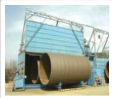
1. Shot blast (External)
