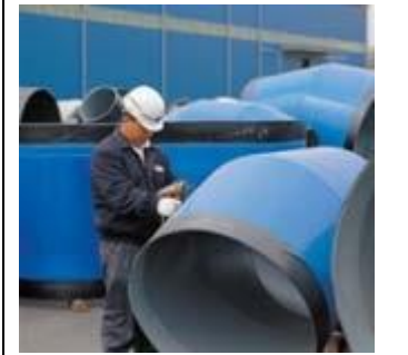
11. External coating thickness measuring
