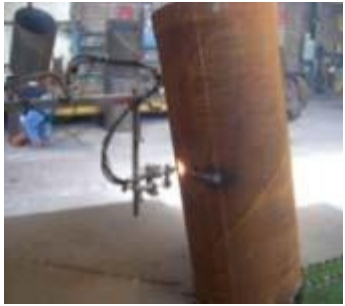
1.Cut fitting in angle
