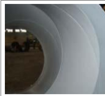
9.FBE & Epoxy coating (Internal surface)
