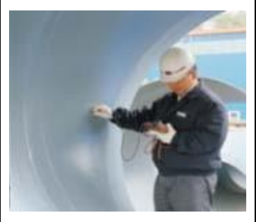
12. Internal coating thickness measuring
