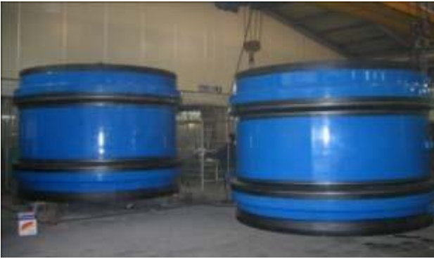
<BELOW FLEXIBLE JOINT>
