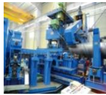
3. Forming & Inside welding
