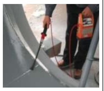
13. Internal pinhole detection
