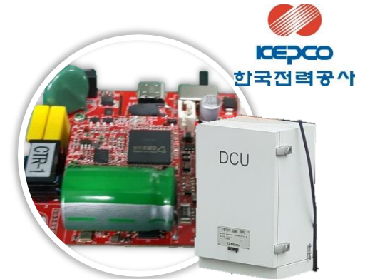
Back-up power for DCU
